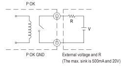
Fig. 2.2 Internal circuit of P OK (Relay, total is 10W)
