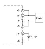
Fig. 3.1 Add on 1~6V external voltage
