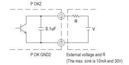
Fig. 2.3 Internal circuit of P OK2 (Open collector method)
